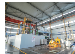
2.5吨VAR真空自耗电弧炉 2.5T VAR vacuum consumable electric arc furnace
