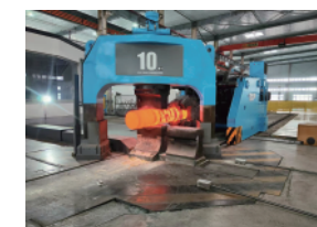
1000-MN 液压机组 1000MN fast forging hydraulic unit
