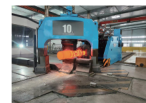
10MN 液压机组 10MN fast forging hydraulic unit
